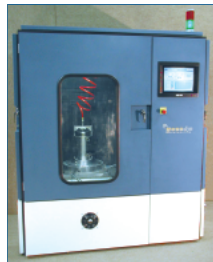
All shook up. Resodyn's equipment uses sonic energy instead of rotors or blades to mix materials.
