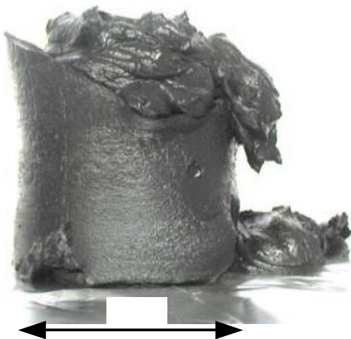
Figure 14. Typical plug of metallized gelled propellant that slid from the reactor vessel.
