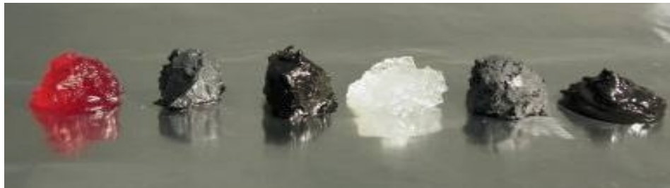
Figure 1. Gelled propellant fuels, both neat and mixed with nano-particles. Pictured from left to right are kerosene, kerosene/nano-aluminum, kerosene/nano-carbon, DMAZ, DMAZ/nano-aluminum, and DMAZ/nano-carbon.
