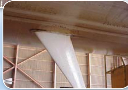
Antenna Cleaned with eOx
